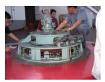
Mechanical Over-speed Device on top of PMG, to be replaced by L&S SSG
